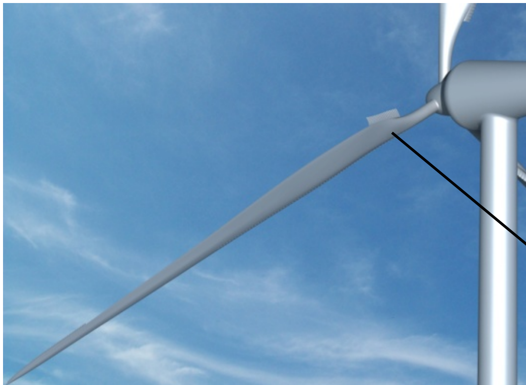
Fig. : Wind turbine blade having a spoiler with effective separation of airflow.
