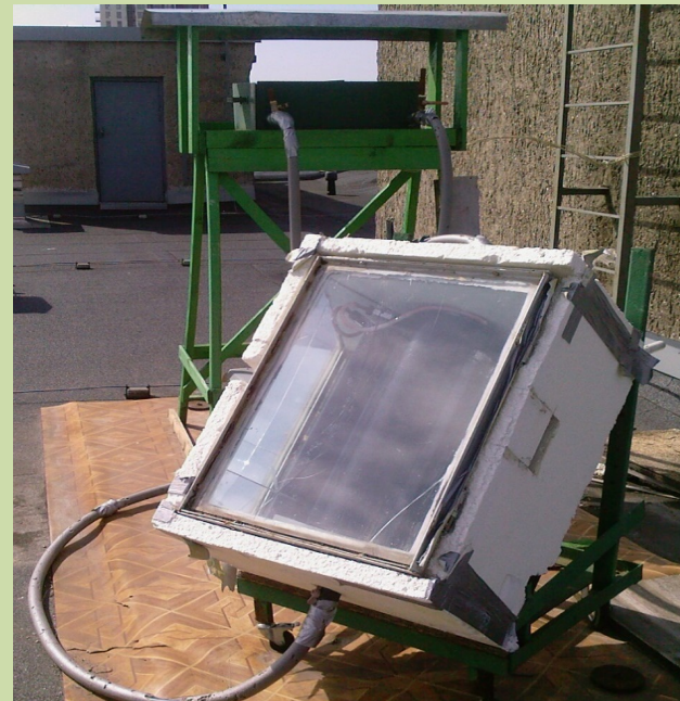
Fig. 2. Heating system scheme: 1 – solar collector; 2 – collector rotation trolley; 3 – heated container/tank filled with artificially contaminated soil; 4 – hoses with additional insulation; 5 – heating element (coil).
